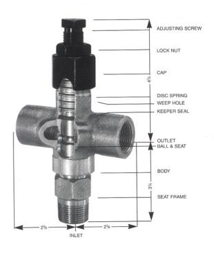
Designed for protection against over-pressure for vessels, pumps, lines, etc. It is a rugged and versatile valve capable of handling a wide range of pressures.
